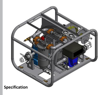
This specification briefly defines the main attributes of a portable helicopter refuelling system. The system is designed for open line refuelling of turbine powered rotary wing and small fixed wing aircraft at flow rates of up to 160 litres / minute using Avtur F34 / Jet – A1 turbine fuels.
